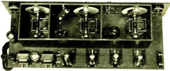
Interior view of the Dar-Mac Supernine. The intermediate frequency amplifier and the audio amplifier extend along the rear of the sub-base.
